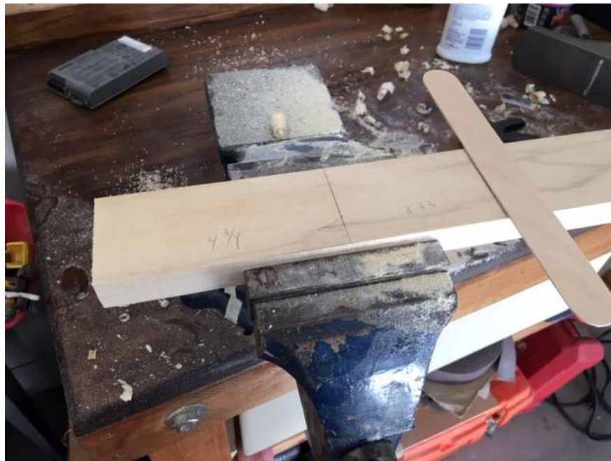
Setup with spacer glued in place and bevel line marked
