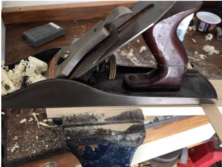
At first, you only cut near the end of the board. As the work progresses, you cut more and more until the bevel reaches the line.
