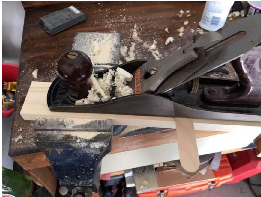
Planing. The spacer tilts the plane up from the work.
