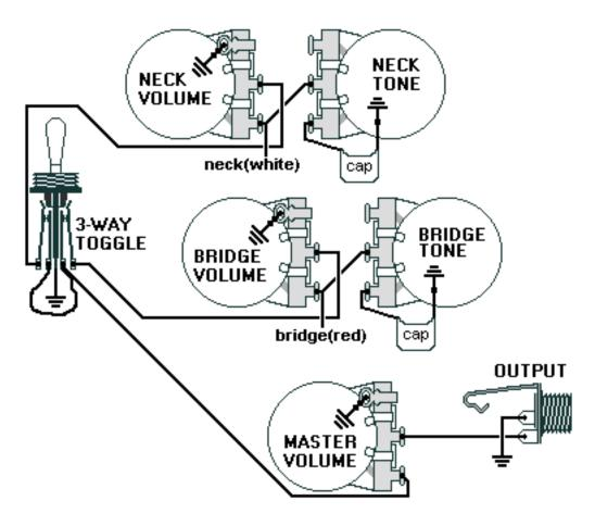
Solder neck (red&green) together and tape up the connection. Solder bridge (black&white together and tape up the connection.
